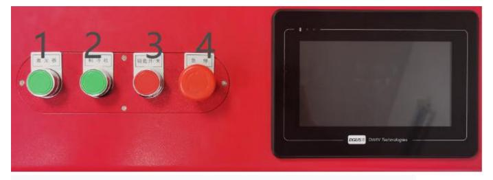
1: laser source; used to control the on and off of the main power
