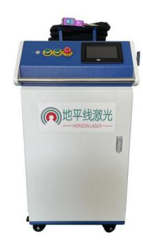
overall design is small, beautiful, and easy to move. It is convenient for customers to choose a working place without being limited by space and scope. This machine can be used for welding applications in billboards, metal doors & windows, sanitary ware, cabinets, boilers, frames and other industries.
