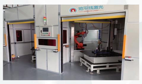
3D robot laser welding machine through the laser control module and the manipulator motion mechanism, match each other and work together. It has a high degree of flexibility and can meet the welding needs of any complex work piece. It is widely used in the automotive industry and electrical cabinet industry.
